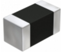
JMK107BJ225KA-T Taiyo Yuden CAP CER 2.2UF 6.3V X5R 0603
