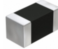
JMK107BJ106MA-L Taiyo Yuden CAP CER 10UF 6.3V X5R 0603
