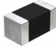
JMK107BJ105KA-T Taiyo Yuden CAP CER 1UF 6.3V X5R 0603
