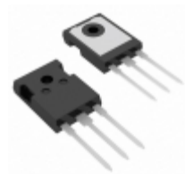
IXGH40N60C2D1 IXYS IGBT 600V 75A 300W TO247AD
