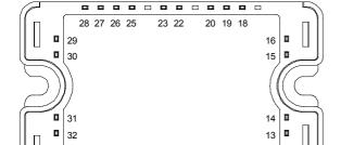
All multiple inputs and outputs must be shorted together Example: 13/14; 29/30; 22/23 ...
