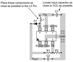
Figure 2. PCB Layout Guide
