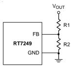
Figure 1. Output Voltage Setting
