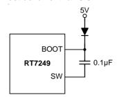
Figure 2. External Bootstrap Diode
