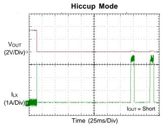
Figure 5. Hiccup Mode Under-Voltage Protection
