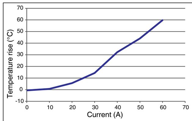
Figure 2 Temperature rise through an FBS bridge (L1 - L1)
