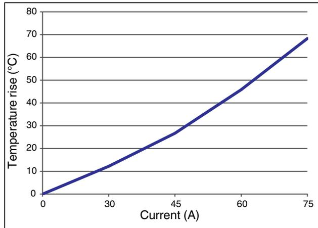
Figure 1 Temperature rise between L0 and L1 across disconnect
