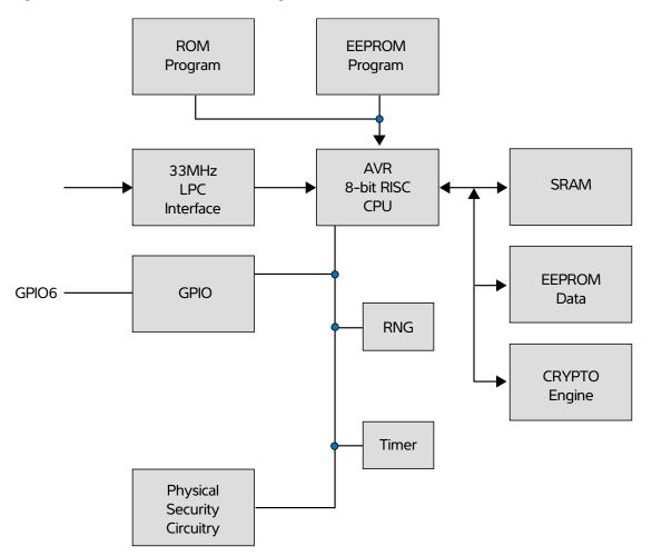
The TPM includes a hardware random number generator, including a FIPS-approved Pseudo Random Number Generator that is used for key generation and TCG protocol functions. The RNG is also available to the system to generate random numbers that may be needed during normal operation.
