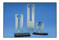
Used to hold and support the THM1SC Harness Mount. The mount is elevated from the harness board so that a cable tie can be installed by Panduit's automatic cable tie installation tools. The mount is pushed into the top of the fixture prior to assembly and pulled out of the fixture when the harness is complete.
