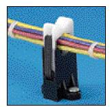
As wires are individually inserted, the bundle is pre-formed. When the harness is complete, it can be easily snapped out. Three sizes available for 1/2" (12.7mm), 3/4" (19.0mm) and 1 1/4" (31.7mm) bundles.
