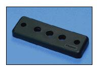
Used with the Harness Board Standoff Post or the Harness Mount Fixture when mounting holes can not be drilled into the harness board. A bolt is inserted from the back side of the adapter and then is turned right side up. The adapter is now ready to be secured to the harness board by using self tapping screws.
