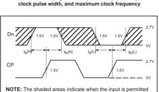
Waveform 2. Data setup and hold times
