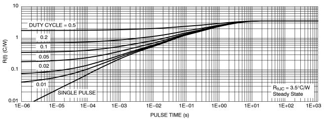
Figure 13. Thermal Impedance (Junction-to-Case) for NDF08N60Z
