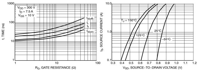
Figure 10. Resistive Switching Time Variation versus Gate Resistance
