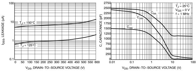
Figure 7. Drain-to-Source Leakage Current versus Voltage
