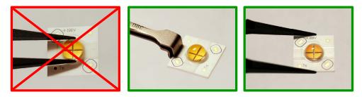
Figure 3. Incorrect handling (left) and correct handling (middle and right) of LUXEON H emitters.
