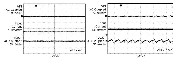
Figure 17. Operating Waveforms in 1x Mode
