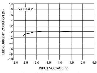
Figure 7. LED Current Change vs. Input Voltage
