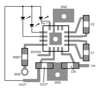
Figure 27. TQFN-16 Recommended Layout
