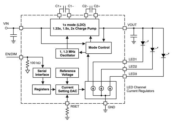
Figure 24. CAT3647 Functional Block Diagram
