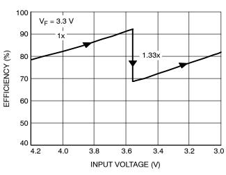
Figure 4. Efficiency vs. Li-Ion Voltage
