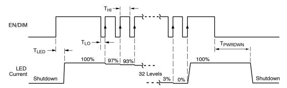
Figure 25. EN/DIM Digital Dimming Timing Diagram
