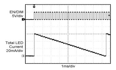
Figure 23. Dimming Waveform
