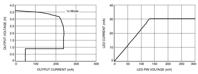
Figure 21. Foldback Current Limit
