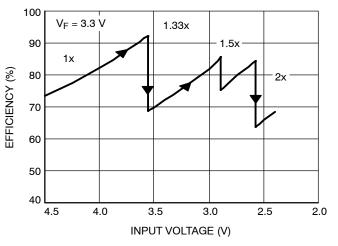
Figure 3. Efficiency vs. Input Voltage
