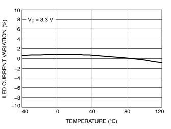
Figure 8. LED Current Change vs. Temperature
