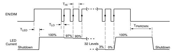
Figure 2. EN/DIM Digital Dimming Timing Diagram
