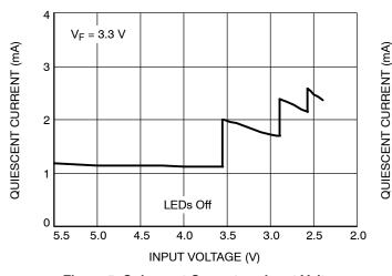
Figure 5. Quiescent Current vs. Input Voltage
