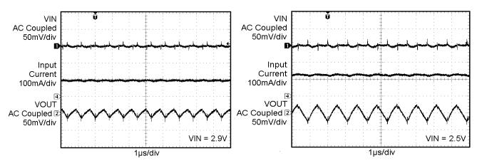
Figure 19. Switching Waveforms in 1.5x Mode
