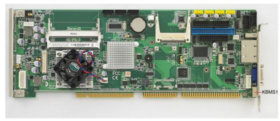
Figure 2.6 PS/2 Keyboard/Mouse Connector (KBMS1)
