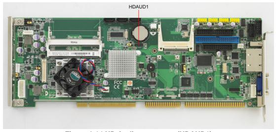
Figure 2.14 HD Audio connector (HDAUD1)
