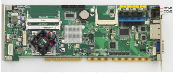
Figure 2.5 Serial Ports (COM1, COM2)
