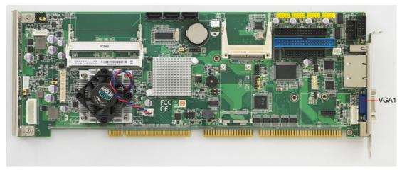
Figure 2.4 VGA Connector (VGA1)
