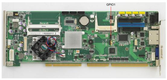
Figure 2.13 GPIO header (GPIO1)
