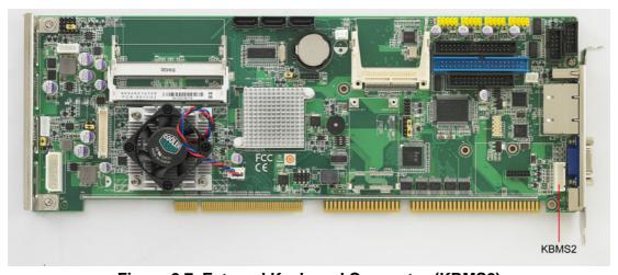
Figure 2.7 External Keyboard Connector (KBMS2)
