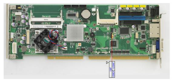
Figure 2.10 Watch Dog Timer (JWDT1) / Infrared (JIR1)/Hardware Monitor Alarm(JOBS1)
