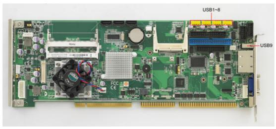
Figure 2.17 USB connector (USB1 to USB8)
