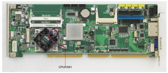
Figure 2.8 CPU Fan Connectors (CPUFAN1)
