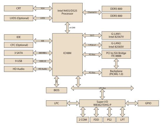
Figure 1.2 Block Diagram
