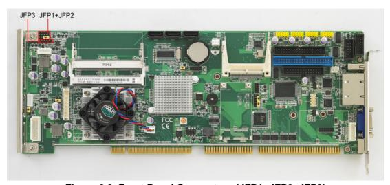
Figure 2.9 Front Panel Connectors (JFP1+JFP2, JFP3)
