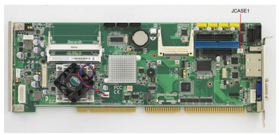
Figure 2.16 JCASE connector (JCASE1)
