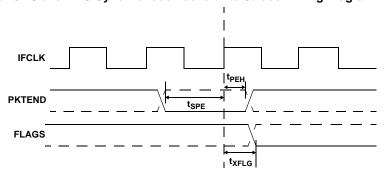
Table 26. Slave FIFO Synchronous Packet End Strobe Parameters with Internally Sourced IFCLK<sup>[25]</sup>
