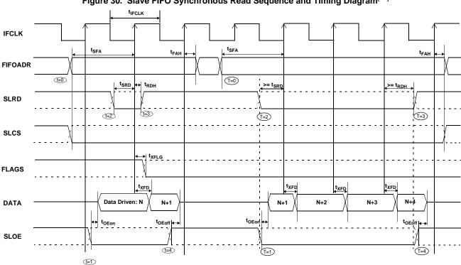
Figure 30. Slave FIFO Synchronous Read Sequence and Timing Diagram<sup>[24]</sup>
