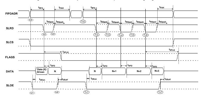
Figure 34. Slave FIFO Asynchronous Read Sequence of Events Diagram
