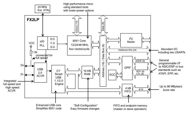
Cypress's EZ-USB<sup>®</sup> FX2LP™ (CY7C68013A/14A) is a low-power version of the EZ-USB FX2™ (CY7C68013), which is a highly integrated, low-power USB 2.0 microcontroller. By integrating the USB 2.0 transceiver, serial interface engine (SIE), enhanced 8051 microcontroller, and a programmable peripheral interface in a single chip, Cypress has created a cost-effective solution that provides superior time-to-market advantages with low power to enable bus-powered applications.
