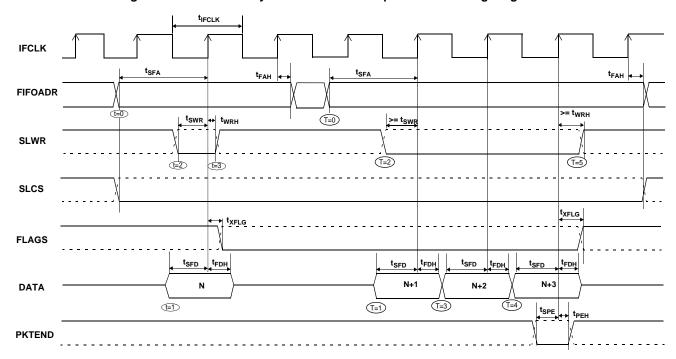
Figure 32 shows the timing relationship of the SLAVE FIFO signals during a synchronous write using IFCLK as the synchronizing clock. The diagram illustrates a single write followed by burst write of three bytes and committing all four bytes as a short packet using the PKTEND pin.
