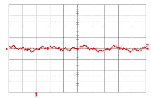
Figure 32. Input reflected ripple current, is (10 mA/div), measured through 10 µH at the source at full rated load current on both outputs and Vin = 48 V. Refer to Fig. 30 for test setup. Time scale: 1 µs/div.
