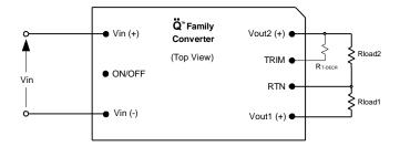
Figure 3. Configuration for decreasing output voltage.
