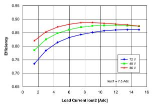
Figure 14. Efficiency vs. load current lout2 and input voltage for converter mounted horizontally with air flowing from pin 3 to pin 4 at a rate of 300 LFM (1.5 m/s), for lout1 = 7.5 A and Ta = 25 C.
