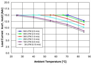
Figure 9. Available balanced load current (lout1 = lout2) vs. ambient air temperature and airflow rates for converter mounted vertically with Vin = 48 V, air flowing from pin 3 to pin 1 and maximum FET temperature ≤ 120 °C.
