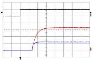
Figure 17. Turn-on transient waveforms at no load current and Vin = 48 V, triggered via ON/OFF pin. Top trace: ON/OFF signal (5 V/div.). Bottom traces: Vout1 (blue, 1 V/div.), Vout2 (red, 1 V/div.). Time scale: 1 ms/div.
