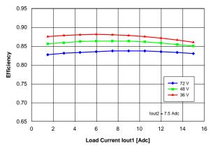
Figure 11. Efficiency vs. load current lout1 and input voltage for converter mounted vertically with air flowing from pin 3 to pin 1 at a rate of 300 LFM (1.5 m/s), for lout2 = 7.5 A and Ta = 25 °C.
