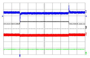
Figure 19. Output voltage response to lout1 load current stepchange of 3.75 A (50%-75%-50%) at lout2 = 7.5 A and Vin = 48 V. Ch1 = Vout1 (50 mV/div), Ch2 = Vout2 (50 mV/div), Ch3 = lout1 (10 A/div.), Ch4 = lout2 (10 A/div.). Current slew rate: 0.1 A/μs, Co = 10 μF tantalum + 1 μF ceramic. Time scale: 0.5 ms/div.
