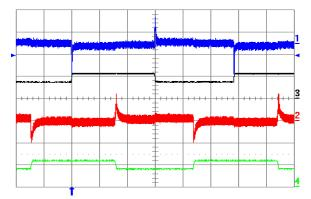
Figure 23. Output voltage response to both lout1 and lout2 (out of phase) load current step-change of 3.75 A (50%-75%-50%) at Vin = 48 V. Ch1 = Vout1 (50 mV/div), Ch2 = Vout2 (50 mV/div), Ch3 = lout1 (10 A/div.), Ch4 = lout2 (10 A/div.). Current slew rate: 0.1 A/μs, Co = 10 μF tantalum + 1 μF ceramic. Time scale: 1.0 ms/div.
