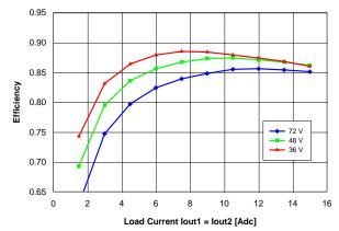
Figure 16. Efficiency vs. balanced load current (lout1 = lout2) and input voltage for converter mounted horizontally with air flowing from pin 3 to pin 4 at a rate of 300 LFM (1.5 m/s) and Ta = 25 °C.
