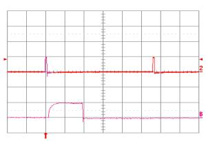
Figure 30. Load current lout2 into a 10 m $\Omega$  short circuit on Vout2 during restart, with Vout1 open (no load), at Vin = 48 V. Ch2 = lout2 (20 A/div, 20 ms/div). ChB = lout2 (20 A/div, 1 ms/div) is an expansion of the on-time portion of lout2.
