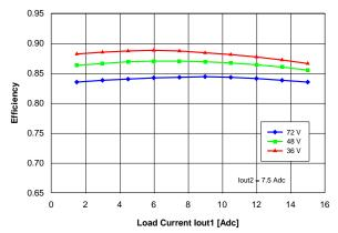
Figure 12. Efficiency vs. load current lout1 and input voltage for converter mounted horizontally with air flowing from pin 3 to pin 4 at a rate of 300 LFM (1.5 m/s), for lout2 = 7.5 A and Ta = 25 °C.
