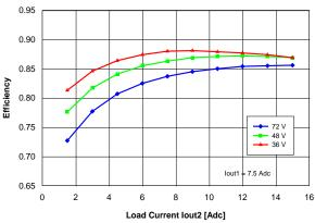
Figure 13. Efficiency vs. load current lout2 and input voltage for converter mounted vertically with air flowing from pin 3 to pin 1 at a rate of 300 LFM (1.5 m/s), for lout1 = 7.5 A and Ta = 25 °C.
