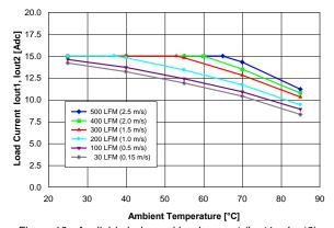
Figure 10. Available balanced load current (lout1 = lout2) vs. ambient temperature and airflow rates for converter mounted horizontally with Vin = 48 V, air flowing from pin 3 to pin 4 and maximum FET temperature ≤ 120 °C.
