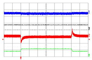
Figure 20. Output voltage response to lout2 load current stepchange of 3.75 A (50%-75%-50%) at lout1 = 7.5 A and Vin = 48 V. Ch1 = Vout1 (50 mV/div), Ch2 = Vout2 (50 mV/div), Ch3 = lout1 (10 A/div.), Ch4 = lout2 (10 A/div.). Current slew rate: 0.1 A/μs, Co = 10 μF tantalum + 1 μF ceramic. Time scale: 0.5 ms/div.
