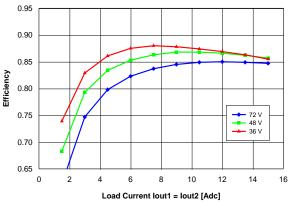
Figure 15. Efficiency vs. balanced load current (lout1 = lout2) and input voltage for converter mounted vertically with air flowing from pin 3 to pin 1 at a rate of 300 LFM (1.5 m/s) and Ta = 25 °C.
