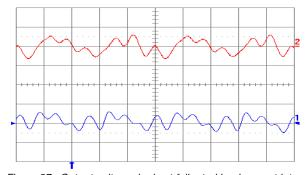
Figure 27. Output voltage ripple at full rated load current into a resistive load on both outputs with Co = 1uF (ceramic) and Vin = 48 V. Ch2 = Vout2, Ch1 = Vout1 (both 20 mV/div). Time scale: 1 μs/div.
