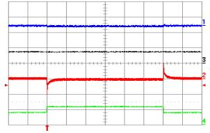
Figure 22. Output voltage response to lout2 load current stepchange of 3.75 A (50%-75%-50%) at lout1 = 7.5 A and Vin = 48 V. Ch1 = Vout1 (100 mV/div), Ch2 = Vout2 (100 mV/div), Ch3 = lout1 (10 A/div.), Ch4 = lout2 (10 A/div.). Current slew rate: 5 A/μs, Co = 300 μF tantalum + 1 μF ceramic. Time scale: 0.5 ms/div.
