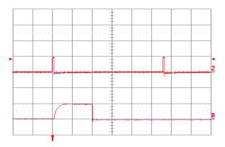
Figure 29. Load current lout1 into a 10 mΩ short circuit on Vout1 during restart, with Vout2 open (no load), at Vin = 48 V. Ch2 = lout1 (20 A/div, 20 ms/div). ChB = lout1 (20 A/div, 1 ms/div) is an expansion of the on-time portion of lout1.
