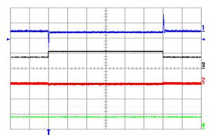
Figure 21. Output voltage response to lout1 load current stepchange of 3.75 A (50%-75%-50%) at lout2 = 7.5 A and Vin = 48 V. Ch1 = Vout1 (100 mV/div), Ch2 = Vout2 (100 mV/div), Ch3 = lout1 (10 A/div.), Ch4 = lout2 (10 A/div.). Current slew rate: 5 A/μs, Co = 300 μF tantalum + 1 μF ceramic. Time scale: 0.5 ms/div.
