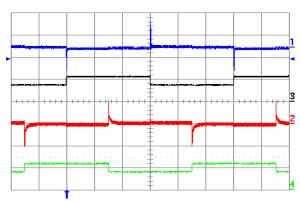
Figure 24. Output voltage response to both lout1 and lout2 (out of phase) load current step-change of 3.75 A (50%-75%-50%) at Vin = 48 V. Ch1 = Vout1 (100 mV/div), Ch2 = Vout2 (100 mV/div), Ch3 = lout1 (10 A/div.), Ch4 = lout2 (10 A/div.). Current slew rate: 5 A/μs, Co = 300 μF tantalum + 1 μF ceramic. Time scale: 1.0 ms/div.
