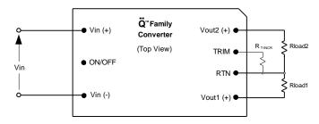
Figure 2. Configuration for increasing output voltage.
