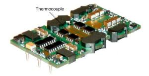
Figure 33. Location of the thermocouple for thermal testing.
