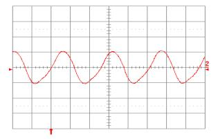
Figure 31. Input reflected ripple current, Ic (100 mA/div), measured at input terminals at full rated load current on both outputs and Vin = 48 V. Refer to Fig. 30 for test setup. Time scale: 1 μs/div.
