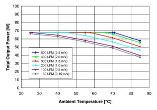
Figure 7. Available output power for balanced load current (lout1 = lout2) vs. ambient air temperature and airflow rates for converter mounted vertically with Vin = 48 V, air flowing from pin 3 to pin 1 and maximum FET temperature ≤ 120 °C.
