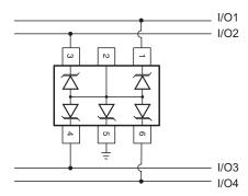
**Bidirection Protection of Four Lines**
